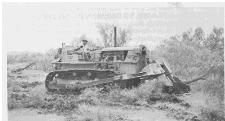
FIGURE 26 Crawler tractor equipped with a stump puller grubbing mesquite in Briscoe County, Texas. (William K. Holt Machinery Co.)
