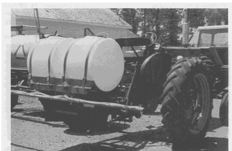
FIGURE 51 Ground spray rig mounted on back of wheel tractor, showing folded boom segments.
